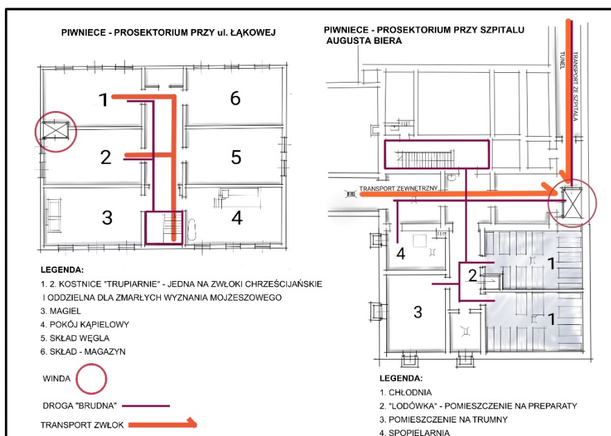
Fig. 2. The prosectorium on Łąkowa Street (left) and the concept for the expansion of the prosectorium at the August Bier Hospital (right), functional diagram of the basements Authors' own illustration based on archival materials 150 .
